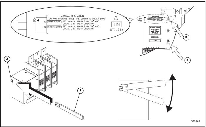
Figure 4-1. Actuating Transfer Switch
