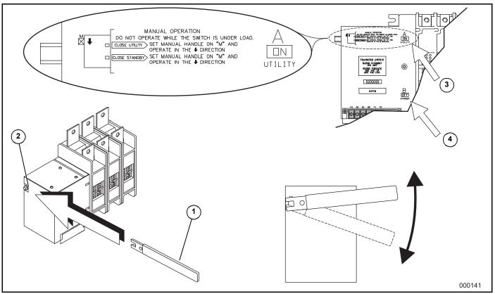
Figure 4-2. Actuating Transfer Switch
