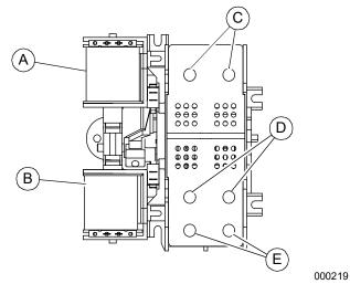
Figure 2-1. Typical Single-Phase ATS Transfer Mechanism
