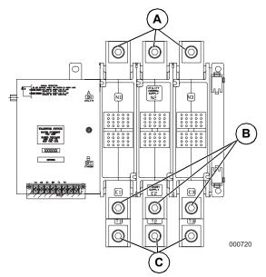
Figure 2-2. Typical Three-Phase 400 Amp Transfer Mechanism
